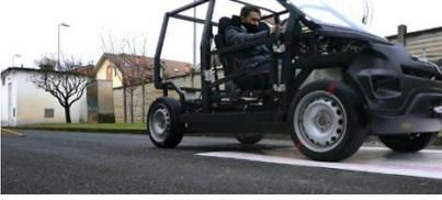
Figure 2: ZEBRA (a) and TELL/Multi-Moby (b) demonstrator vehicles during traction control tests with suddenly varying tyre-road friction conditions, while using the V2X-enabled pre-emptive traction controller.
