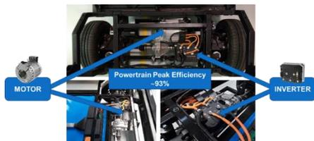
Figure 8: DANA TM4 highly efficient and cost effective medium-voltage (100Vdc) power train integrated in the TELL vehicle
