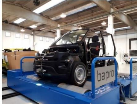
Figure 9: Energy efficiency testing of the TELL vehicle on the rolling road at I-FEVS
