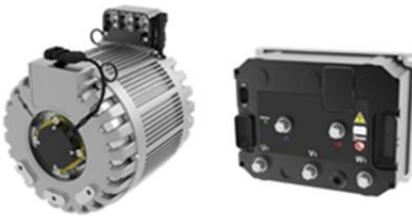
Figure 4: The newly designed motor and inverter from DANA TM<sub>4</sub>, for the 4WD vehicle demonstrator. The inverter testing recorded a 98.8% of peak and a 97.4% of average efficiencies.
