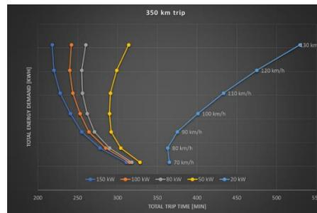
Figure 10: Generic chart of trip time for 350 km as function of vehicle speed and available charging power.
