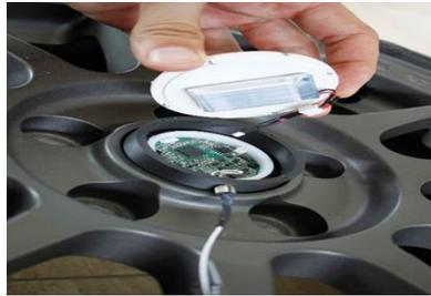
Figure 5: The in-wheel energy harvesting device offers the possibility to transmit signals, sensed in the wheel, with very high data rates to a controller at the chassis.
