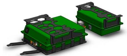
Figure 7: CAD drawing of SELFIE battery pack with cradle
