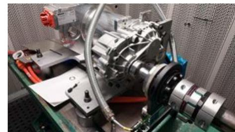
*Figure 8: FITGEN Prototype #1 (transmission and motor-inverter group, stand-alone and mounted on the test-bench, courtesy of FITGEN consortium).*
