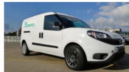
Figure 3: Fiat Doblo (N1) with in-wheel motors in the front and close-to-wheel damping system ready to be evaluated
