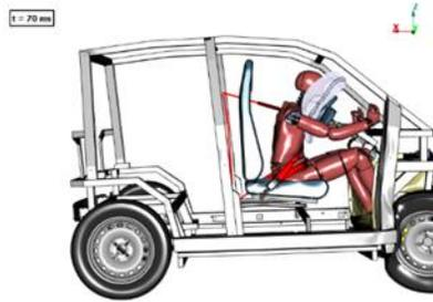
Figure 11: analysis of the restraint system under the R137 crash
