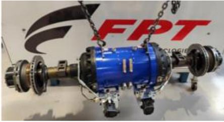
**Figure 4:** Electrical fully modular e-axle for N2-type vehicle ready to be integrated into the IVECO daily demonstrator
