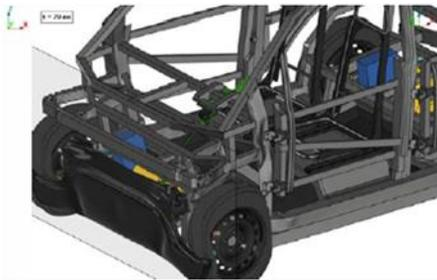
Figure 10: Simulation results of the Multi-Moby vehicle under the R137 crash, after structure optimization
