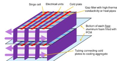
Figure 2 Battery housing structure
