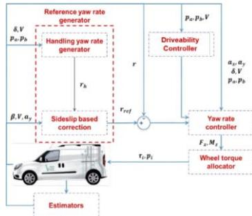
Figure 5 Simplified block diagram of the torque-vectoring control structure
